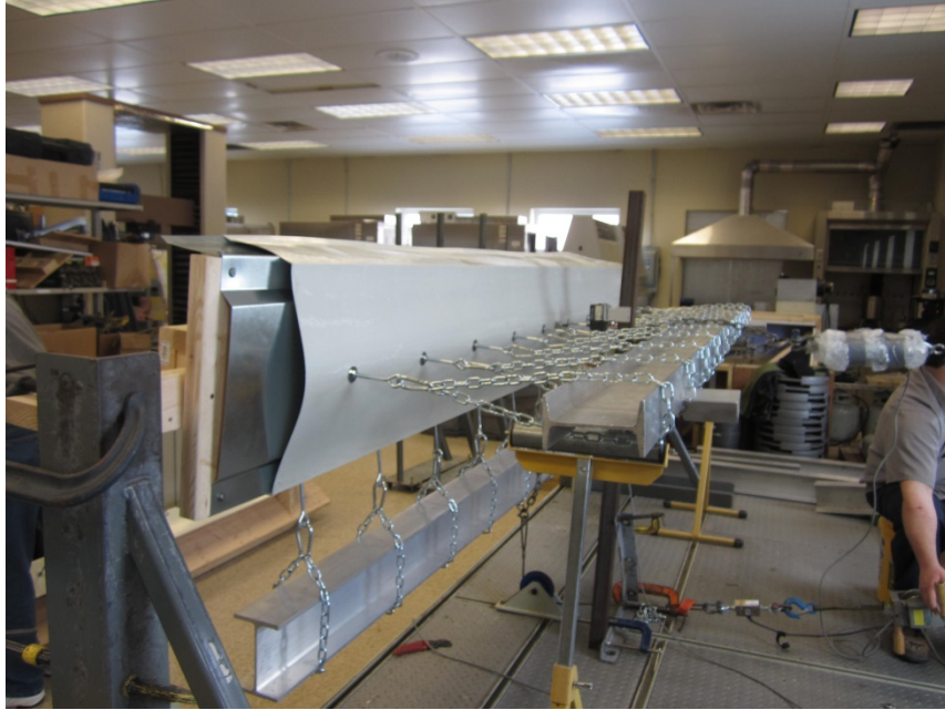
Photo No. 1 Typical SPRI Test RE-3, Coping Pull-Off Test Setup
