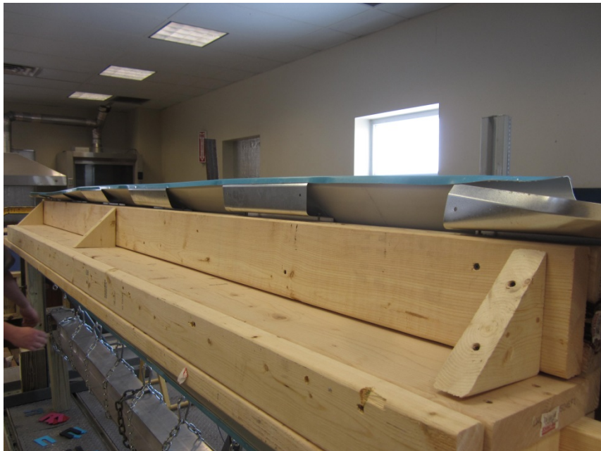
Photo No. 2 Typical SPRI Test RE-3 Mode of Failure; Cleat Failure During Load Application
