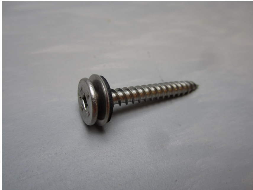
Photo No. 5 Typical Coping Cleat Fastener
