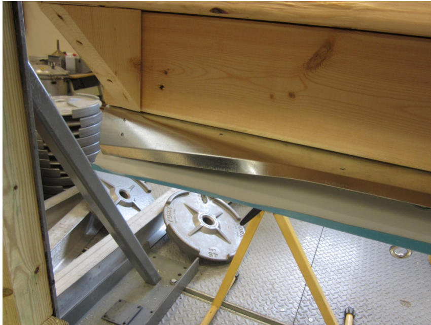
Photo No. 3 Typical SPRI Test RE-3 Mode of Failure; Cleat Failure During Load Application
