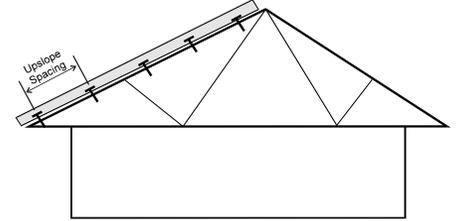
**Grandrib 3** - screws spaced 9" c/c across width (see diagram) X up-slope spacing (see above)
